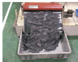
Grinding sludge generated by manufacturing processes
