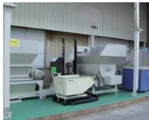
▲ Sludge solidification equipment at the KOFU Plant
