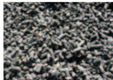
▲ "Iron plastic briquettes" made from grinding swarf
