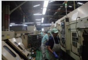
LED lights on the production line are equipped with motion sensors.
