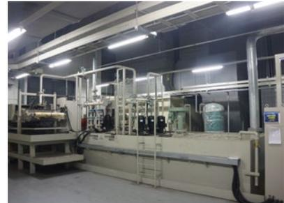
Newly installed semi-centralized coolant tank
