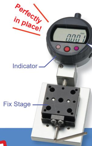
After the position has been adjusted, no movement can be seen on the indicator scale even when the face of the stage is grabbed and forcefully shaken.
