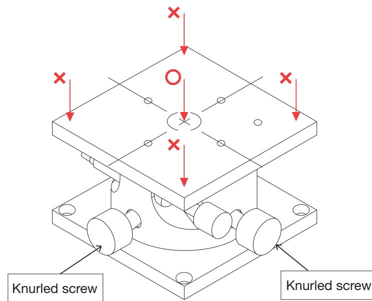
The center of gravity for samples loaded on the tilt/rotary stage should be positioned toward the stage surface center as per the figure above.
