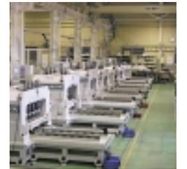
Durability testing devices for determining reliability of LM guides
